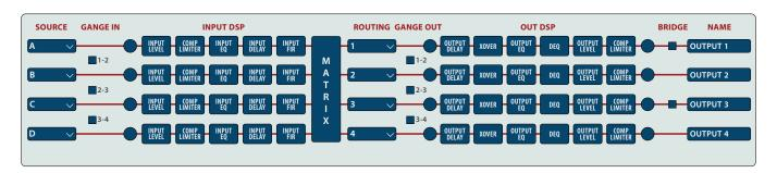
The **PRONET AX control software**, working on a solid and reliable CANBUS based network protocol, provides an intuitive interface for the remote control of the whole audio system via the rear panel etherCON RJ45 connectors, with the possibility to setting all processing parameters and monitoring the status of the amplifier.
